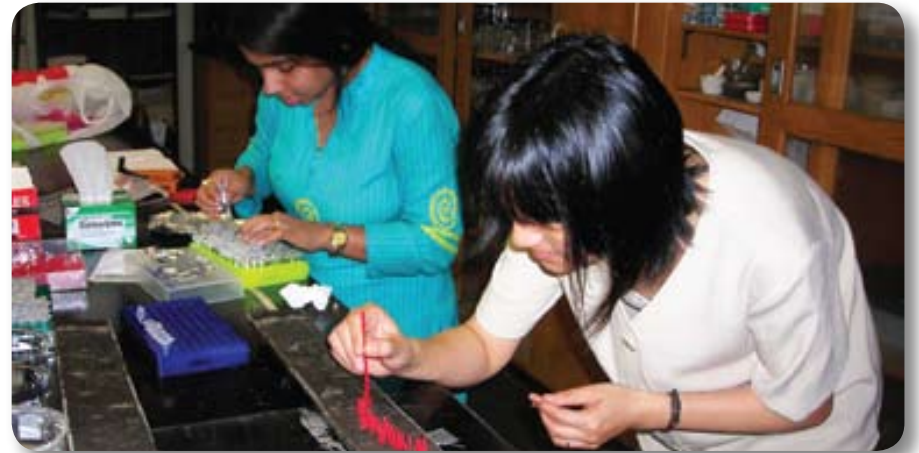
Researchers are conducting isotope sampling along the length of the sediment core every 2mm.
